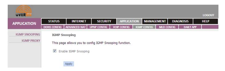
**Enable IGMP Snooping:** Check the box to enable IGMP Snooping of your ONU.
